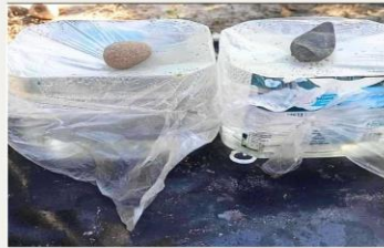
Gallons with plastic bottle inside collecting dews condensed from seawater
