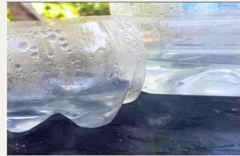
Gallons with plastic bottle inside collecting dews condensed from seawater
